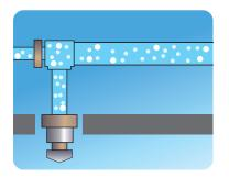
Under the conventional method, since the piping is flushed with air still remaining inside, the residual air is compressed by the pressurized water during flushing, resulting in a large amount of oxygen dissolving in the pressurized water. The dissolved oxygen leads to the corrosion of the piping as time passes.
