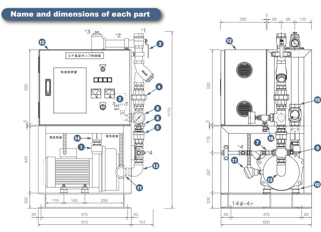
\*1 Connect the SP drain pipe. (40A) \*2 Discharge into the water tank. (40A) \*3 Pour in 4L of pump-priming water initially. \*4 It will sink fire extinguishing water tank(15A) Note: Height must be within 2m down to the water surface of the tank.
