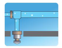
Under the SP vacuum pump method, the piping can be flushed in a vacuum state because the air remaining in the piping until the sprinkler head is removed by the strong suction power of the pump. This prevents an increase in the amount of dissolved oxygen, thereby protecting the piping from corrosion.
